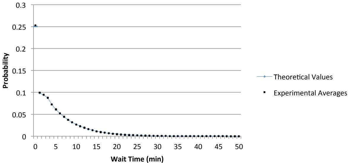
Figure 1: A comparison of the theoretical and experimental probability distributions for average customer wait time on a 150 customer day with only one server available. Notice that the two graphs match each other almost exactly, indicating that our computational simulation has a high accuracy when run over 10,000 trials. The only significantly visible error is the slightly higher experimental value for wait time 0.
