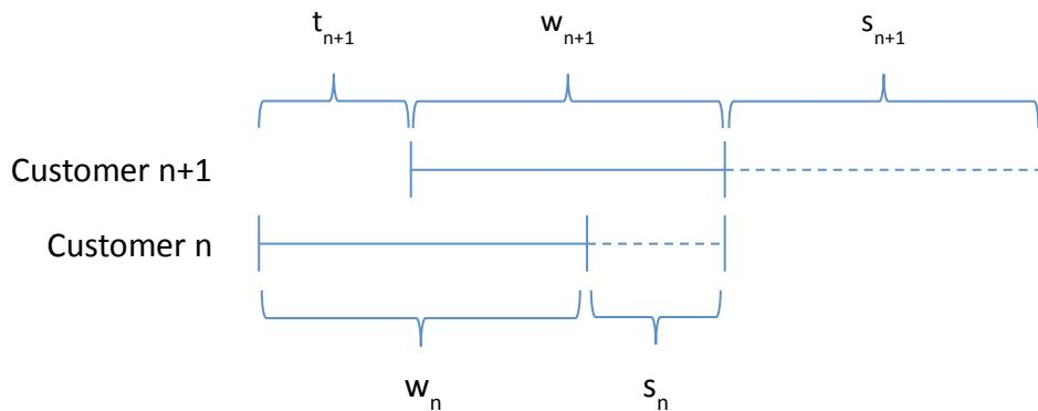
Figure 2: A diagram illustrating the derivation for the value of  $w_n$  given  $w_{n-1}$ ,  $s_{n-1}$ , and  $t_n$ .
